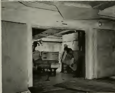
Bottom, left: View of one of 20 huge refrigerator compartments for perishable cargo on the newly reconverted vessel. It cost Matson $750,000 to reconvert this vessel to meet the requirements of the Hawaiian trade.
